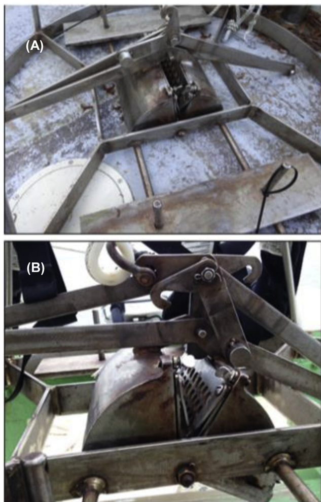
Fig. 5. (A) Top and (B) side views of the Young Grab used in sediment samplings.
