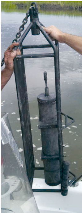
Fig. 2. Long-term acoustic recorders (DSG-Ocean) were deployed on the bottom of the May River. DSG-Ocean recorders in frames to minimize noise artifacts and impacts on the instruments
